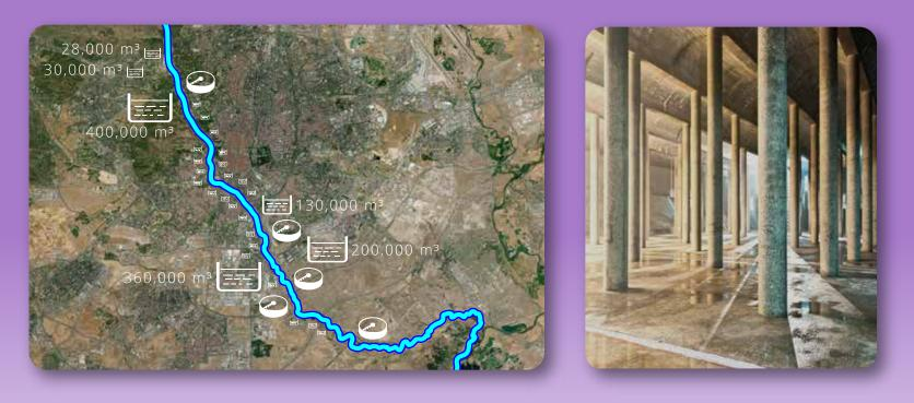
The main advantage is that sewage can be distributed along different paths, which allows certain level of freedom to redirect sewage between different tanks. In this way overflowing or flooding will not happen.
