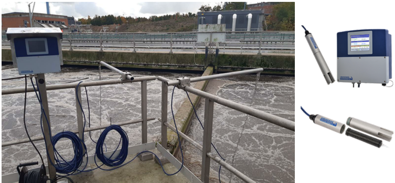
Figure 8 Liquid phase N_2O Wastewater System sensor body, head and panel and in-situ (Unisense Environment).
